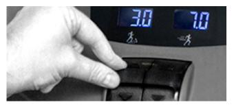
**Step 5:** Begin pedaling. Adjust the left motion control to change the incline level.
